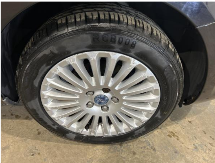
1: Wheel osf Scratched Over 50mm
