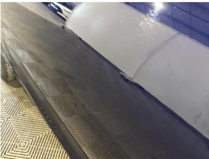
7: Door nsf Dented Between 10mm + 30mm
