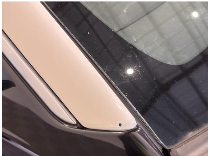
18: A Post os Chipped 1 To 5
