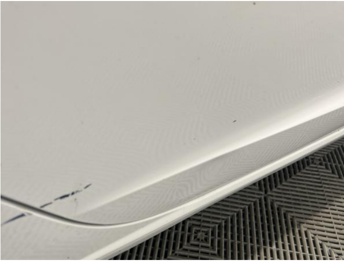
3: Door osr Scratched Over 25mm Not Thru Paint
