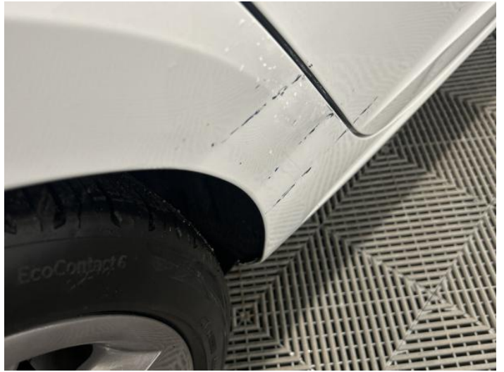
4: Qtr Panel osr Dented With Paint Damage
