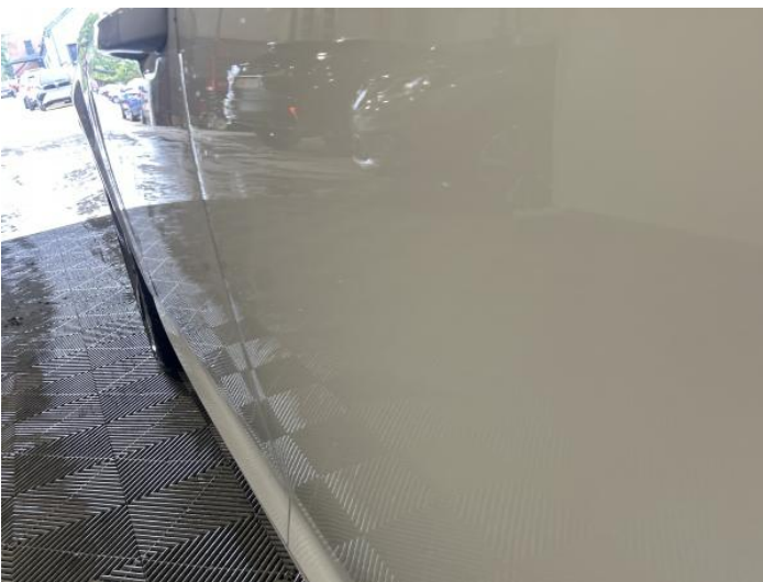
7: Door nsr Dented Between 10mm + 30mm
