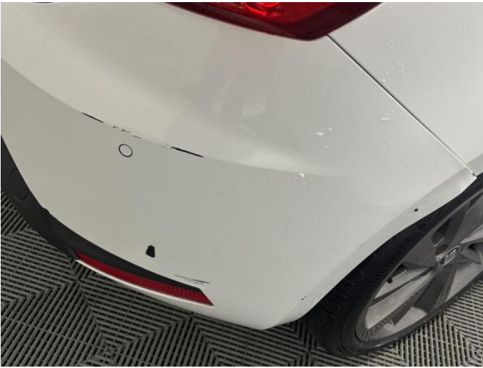
5: Bumper Rear Scratched 25 to 100mm Thru Paint
