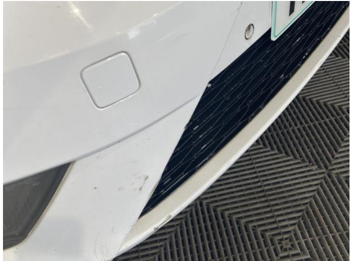
10: Bumper Front Scratched Over 100mm Thru Paint
