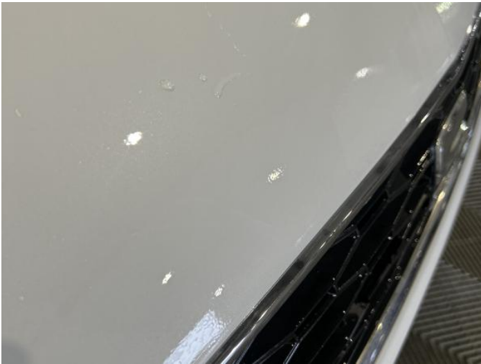
11: Bonnet Poor Previous Repair Poor Paint
