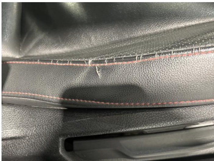
15: Seat Base Cover osf Torn UpTo 3mm
