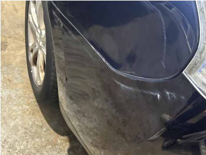
9: Bumper Rear Scratched Over 100mm Thru Paint
