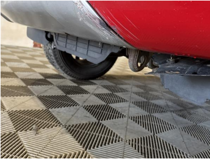
3: Bumper Front Moulding Broken Replace
