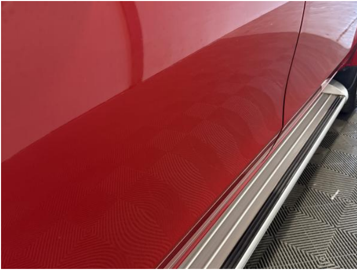
9: Door osr Poor Previous Repair Poor Paint
