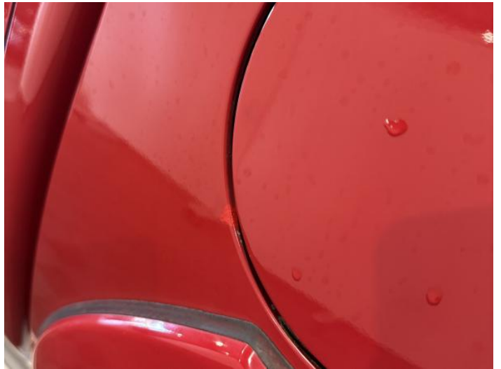
6: Qtr Panel nsr Chipped Over 5mm
