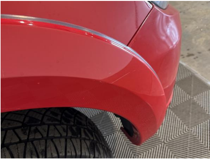
11: Wing Front Arch Extension os Scratched (Painted) Over 25mm Thru Paint
