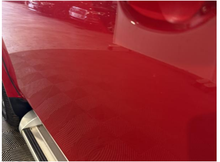
4: Door nsf Dented Between 10mm + 30mm
