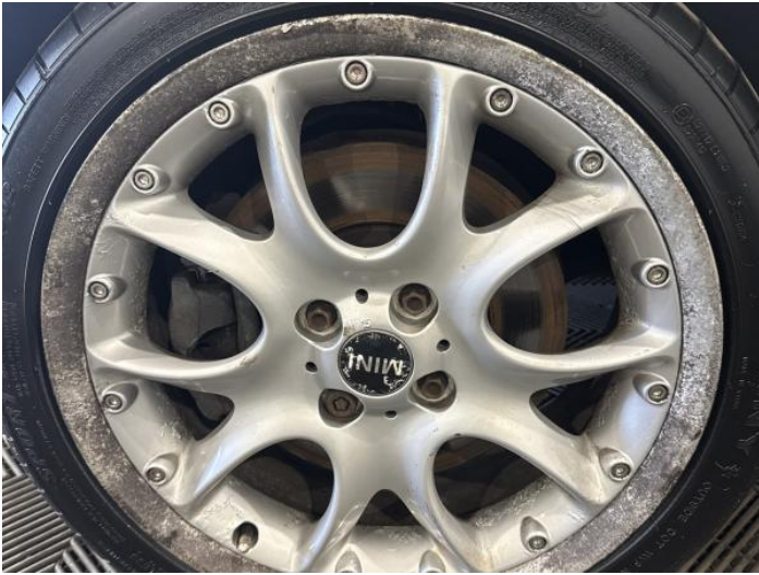
3: Wheel nsf Scratched Over 50mm
