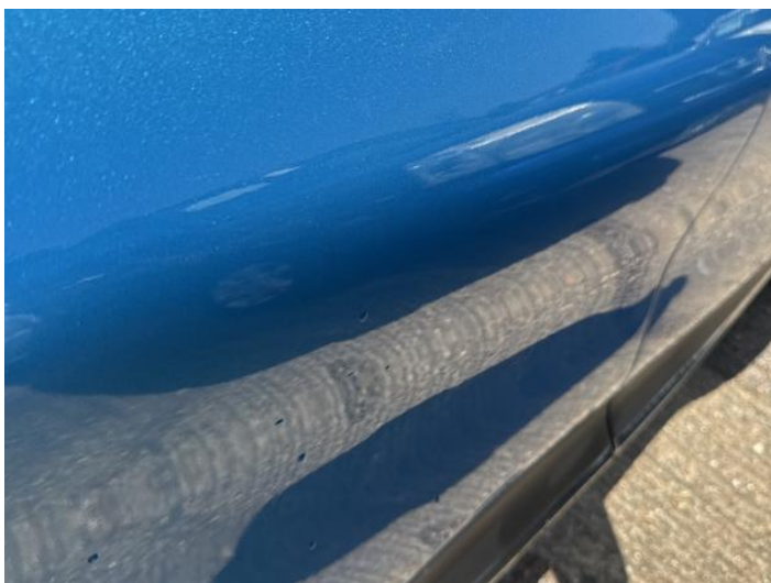
5: Door osr Dented Over 2 UpTo 10mm
