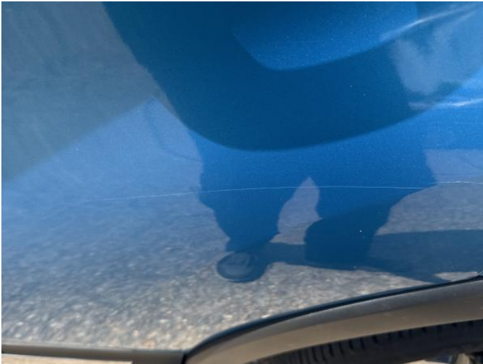
15: Door nsr Scratched Over 25mm Thru Paint
