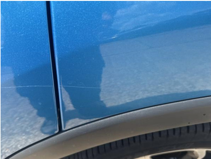
17: Qtr Panel nsr Scratched Over 25mm Thru Paint
