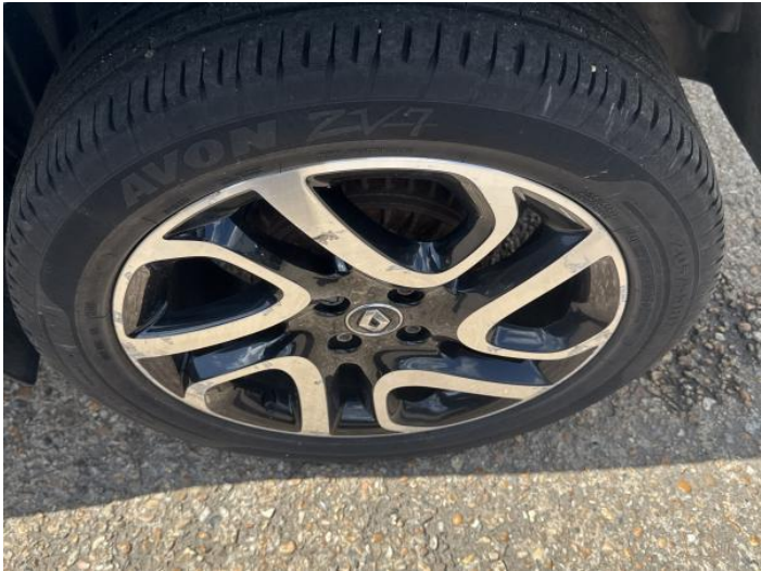
16: Wheel nsr Scratched Over 50mm
