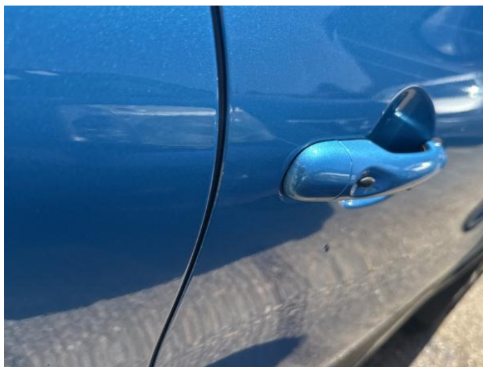
6: Door osr Dented Over 2 UpTo 10mm
