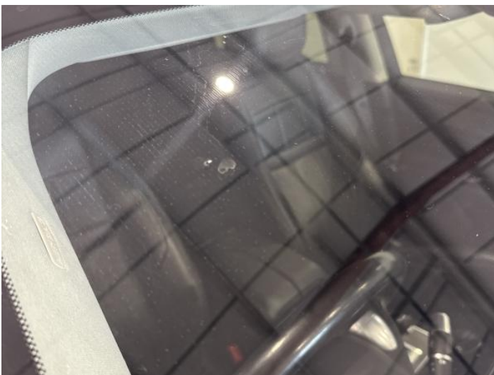
13: Screen Front Chipped UpTo 10mm
