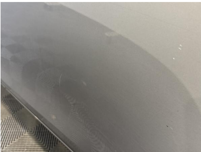
7: Door nsr Scratched Over 25mm Thru Paint
