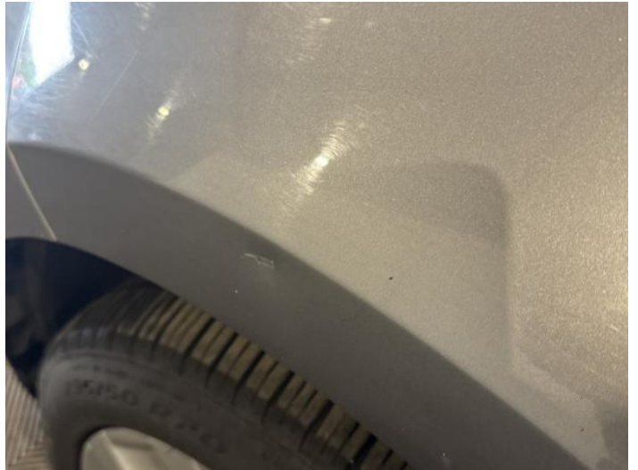
4: Wing nsf Scratched UpTo 25mm Thru Paint
