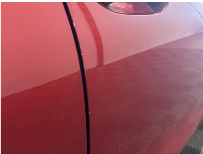
7: Door osf Chipped Edge Chip
