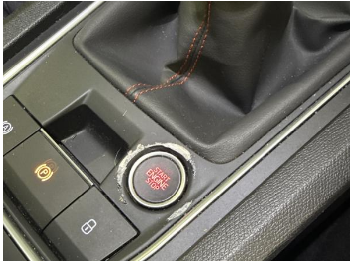
10: Centre Console Front Scuffed UpTo 25mm
