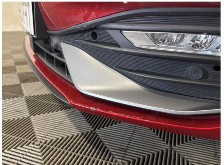
2: Bumper Front Scratched UpTo 25mm Thru Paint
