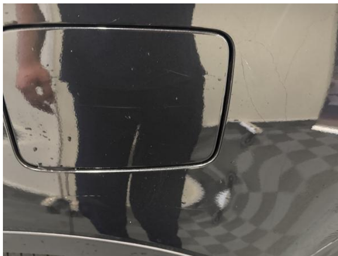
10: Qtr Panel nsr Dented With Paint Damage
