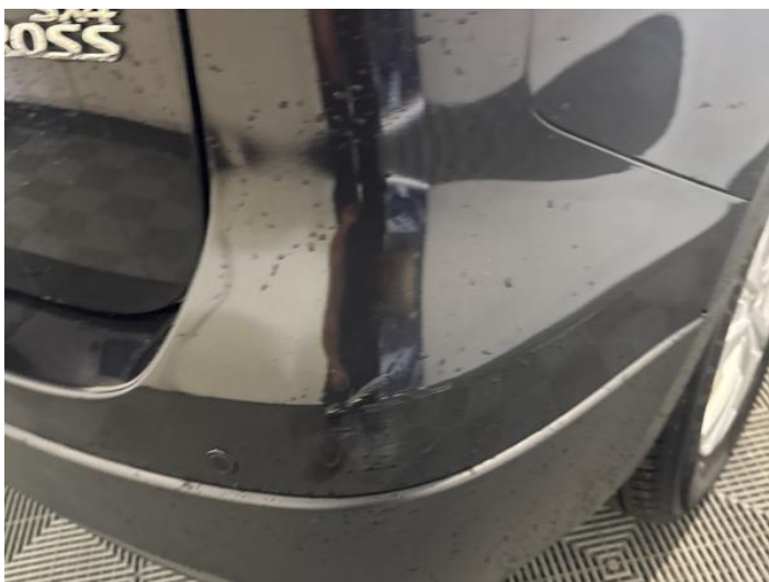
11: Bumper Rear Scratched Over 100mm Thru Paint
