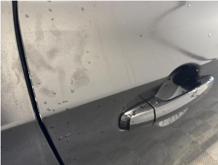
15: Door osr Poor Previous Repair Poor Paint
