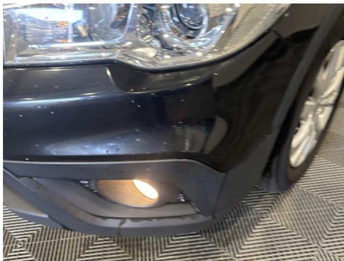
2: Bumper Front Scratched 25 to 100mm Thru Paint
