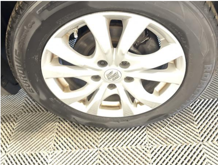
17: Wheel osf Scratched Over 50mm
