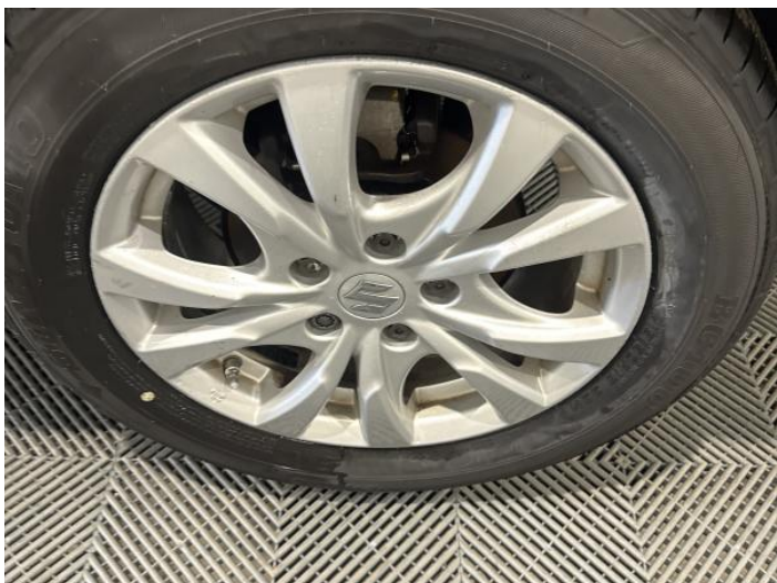
9: Wheel nsr Scratched Over 50mm
