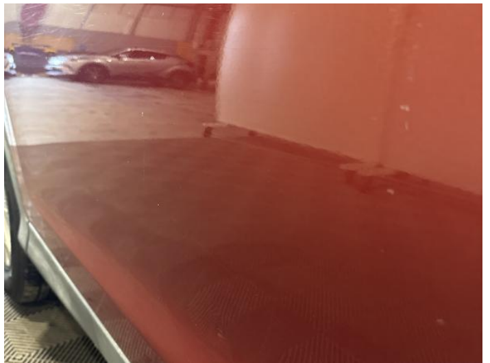
6: Door nsf Scratched Over 25mm Thru Paint
