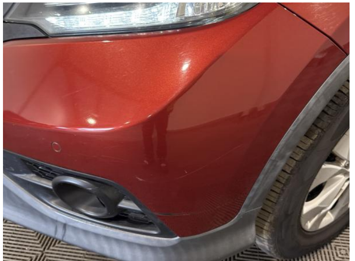
2: Bumper Front Scratched Over 100mm Thru Paint
