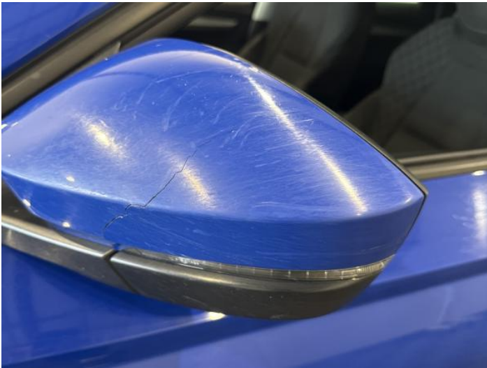
5: Door Mirror Assy nsf Broken Replace
