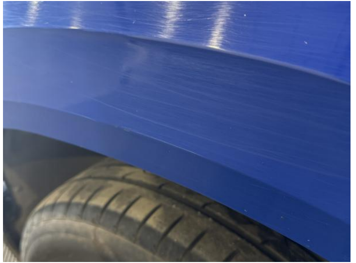
4: Wing nsf Scratched Over 25mm Thru Paint
