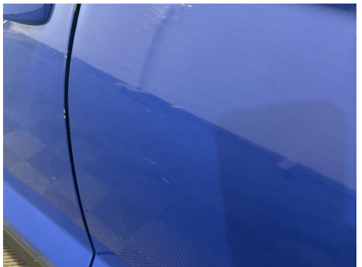
8: Door nsr Scratched Over 25mm Thru Paint
