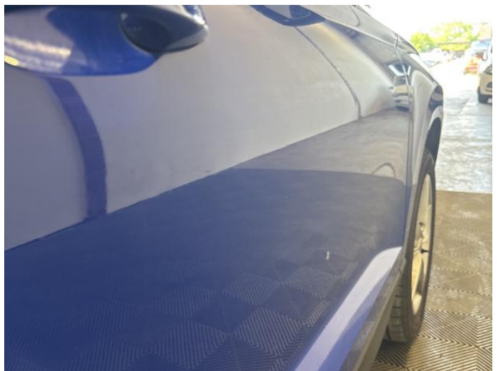
14: Door osf Dented Over 30mm
