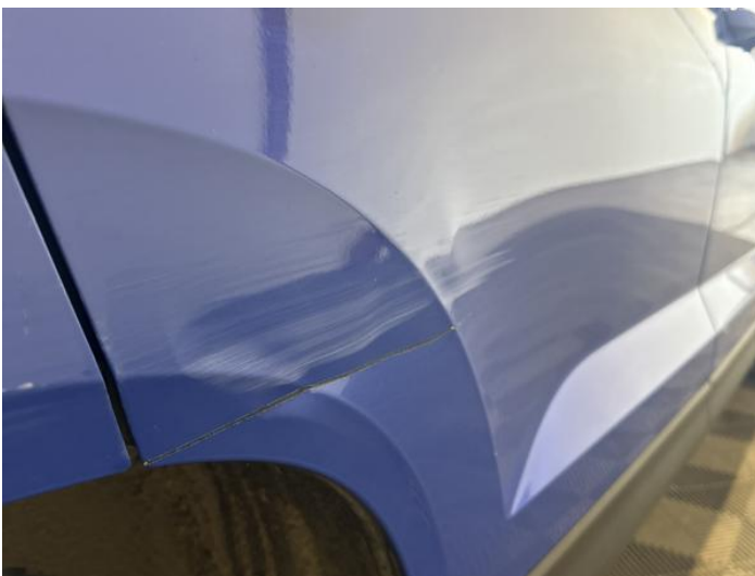
13: Door osr Dented With Paint Damage
