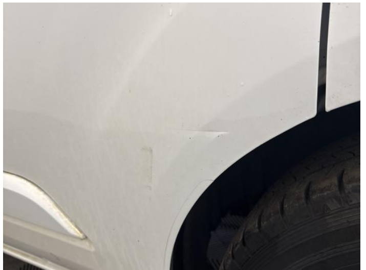
18: Door osf Dented With Paint Damage
