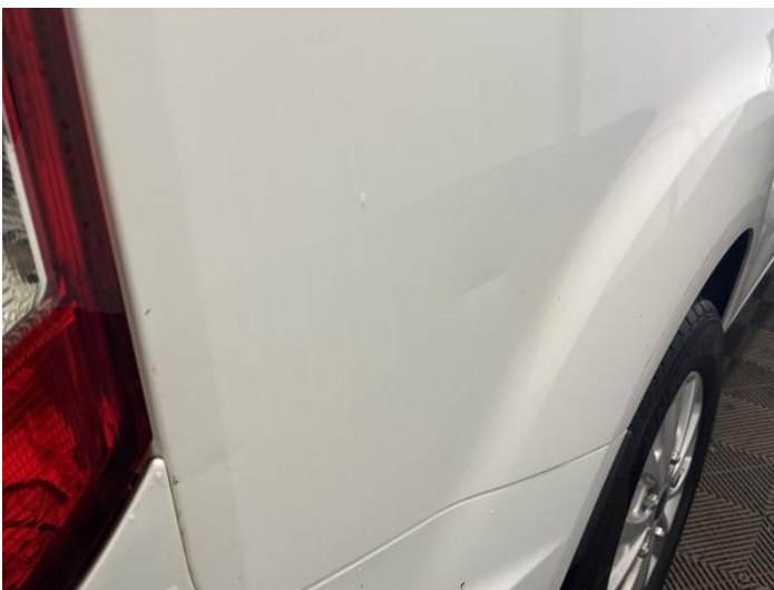
13: Qtr Panel osr Dented With Paint Damage
