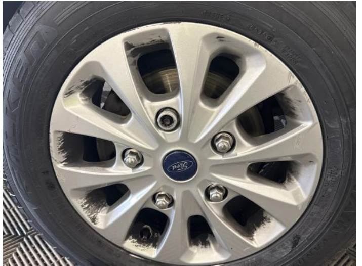
4: Wheel nsf Scratched Over 50mm
