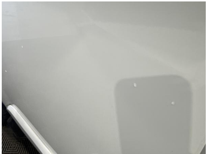
6: Door nsf Dented Between 10mm + 30mm
