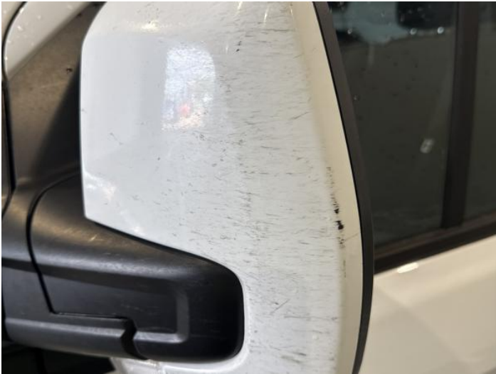
3: Door Mirror Assy Scratched (Painted) Over 25mm Thru Paint
