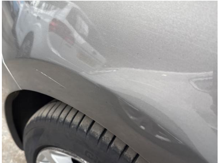
4: Wing nsf Scratched Over 25mm Thru Paint
