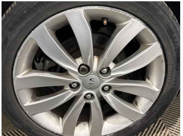
12: Wheel osr Scratched Over 50mm
