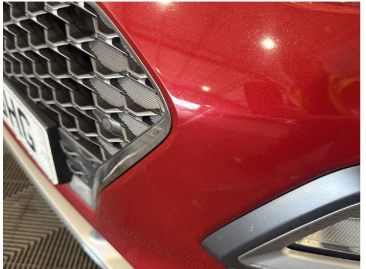
2: Bumper Front Scratched 25 to 100mm Thru Paint
