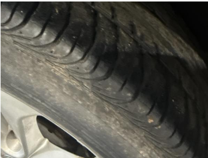
11: Tyre nsr Damaged Replace
