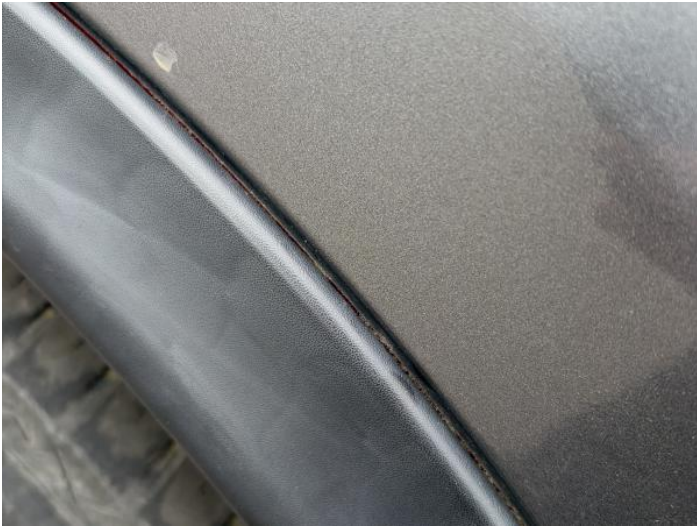
9: Wing nsf Scratched UpTo 25mm Thru Paint
