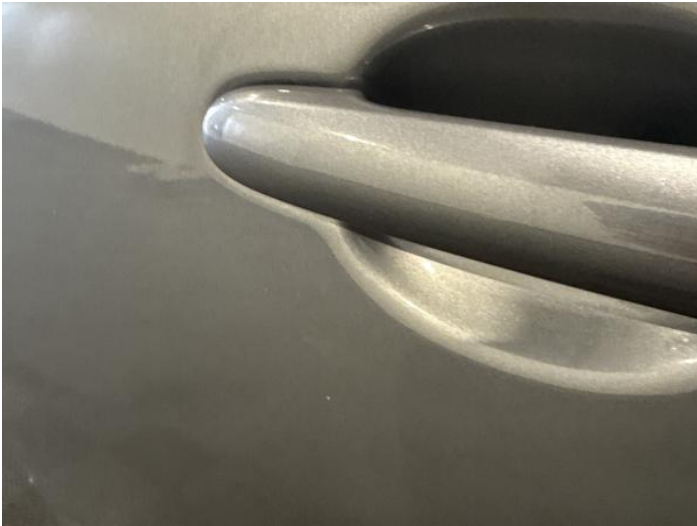
3: Door nsf Scratched UpTo 25mm Thru Paint
