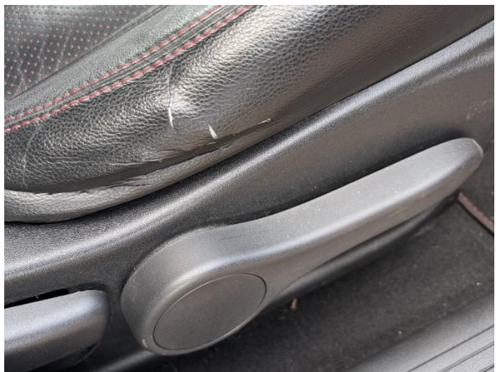
8: Seat Base Cover osf Torn UpTo 3mm
