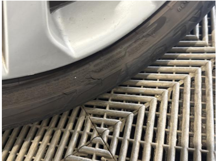
10: Tyre osf Damaged Replace
