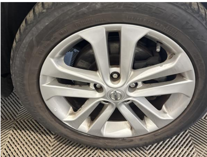
7: Wheel osf Scratched Over 50mm
