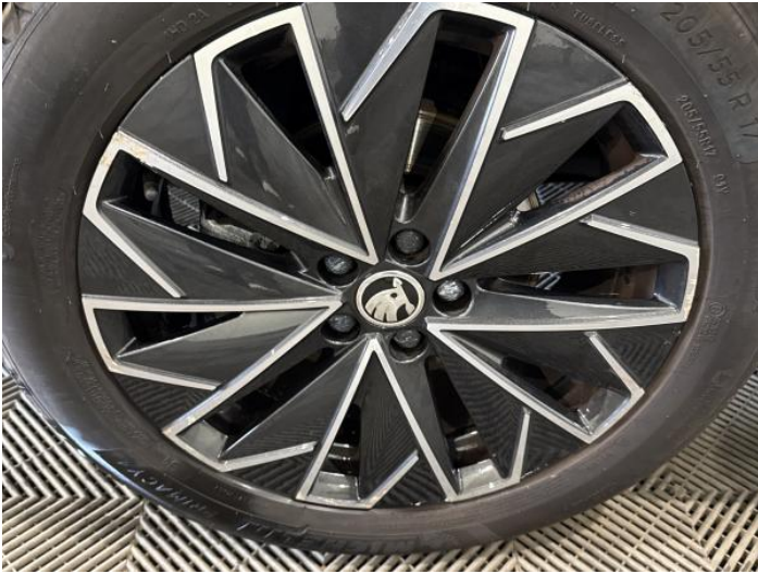
3: Wheel nsf Scratched Over 50mm
