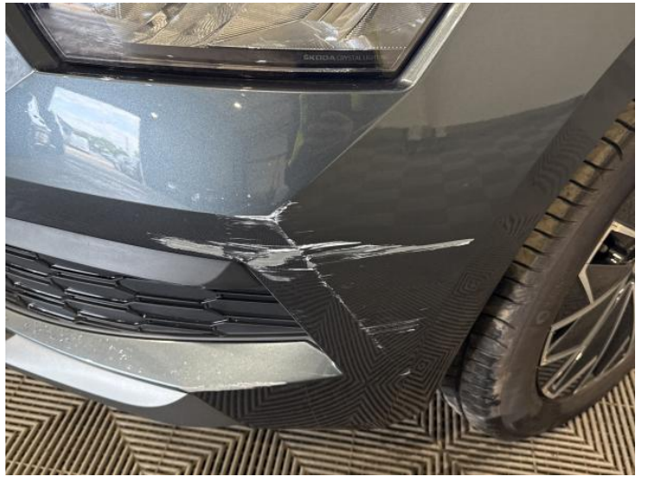
2: Bumper Front Scratched 25 to 100mm Thru Paint
