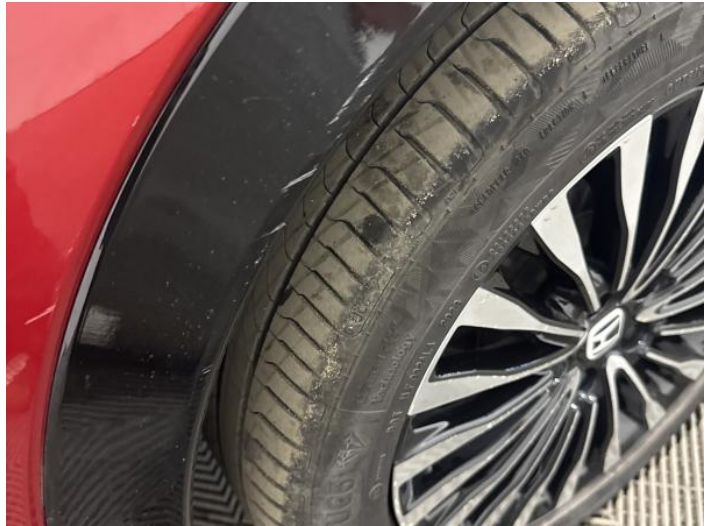
10: Qtr Panel Arch Extension os Scratched (Painted) Over 25mm Thru Paint
