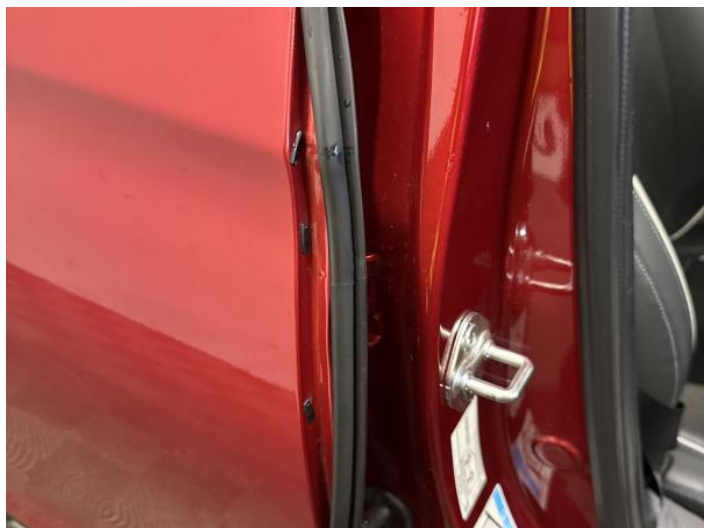
8: Aperture Seal osr Broken Replace
