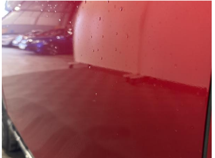
4: Door nsf Poor Previous Repair Poor Paint
