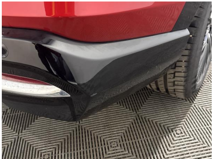
6: Bumper Rear Moulding Scratched (Painted) Over 25mm Thru Paint
