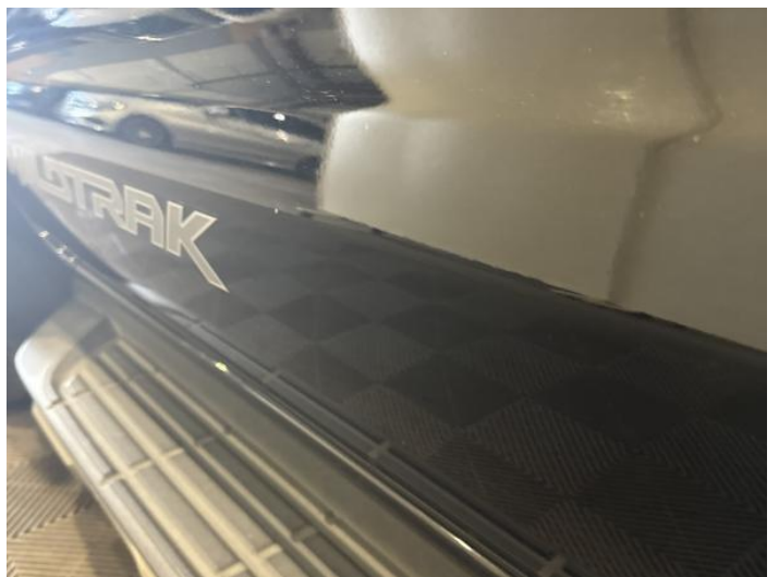
8: Door nsf Chipped 1 To 5
