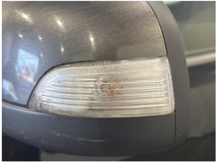
6: Flasher Side Repeater ns Broken Replace
