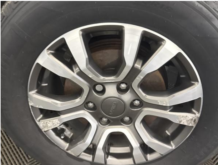
17: Wheel osr Corroded Light
