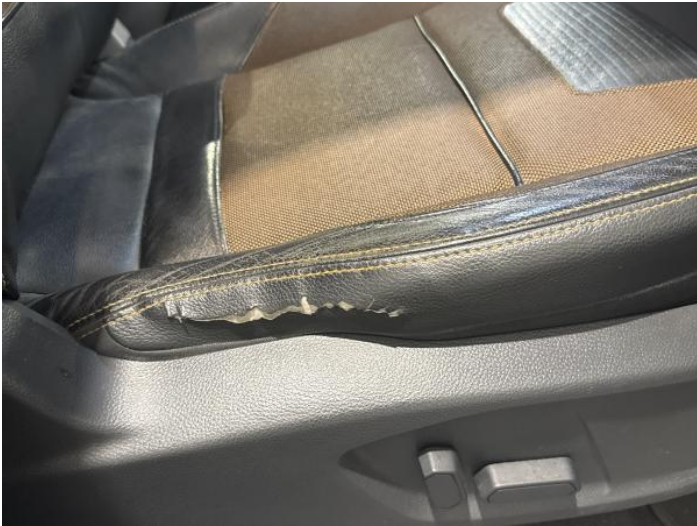
21: Seat Base Cover osf Torn Over 3mm
