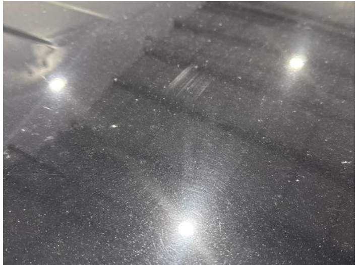
22: Roof Scratched Over 25mm Thru Paint
