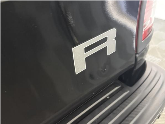
15: Tailgate Dented With Paint Damage
