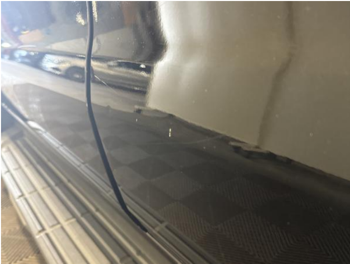
9: Door nsr Dented Between 10mm + 30mm
