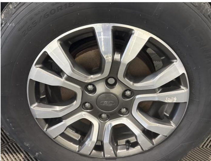
13: Wheel nsr Corroded Light
