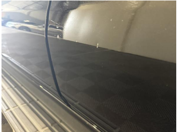
10: Door nsr Scratched Over 25mm Thru Paint
