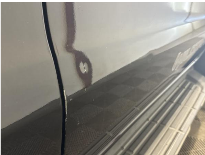
19: Door osf Dented With Paint Damage
