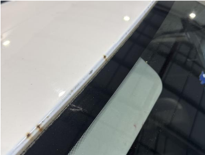
21: Roof Rusted Over 5mm
