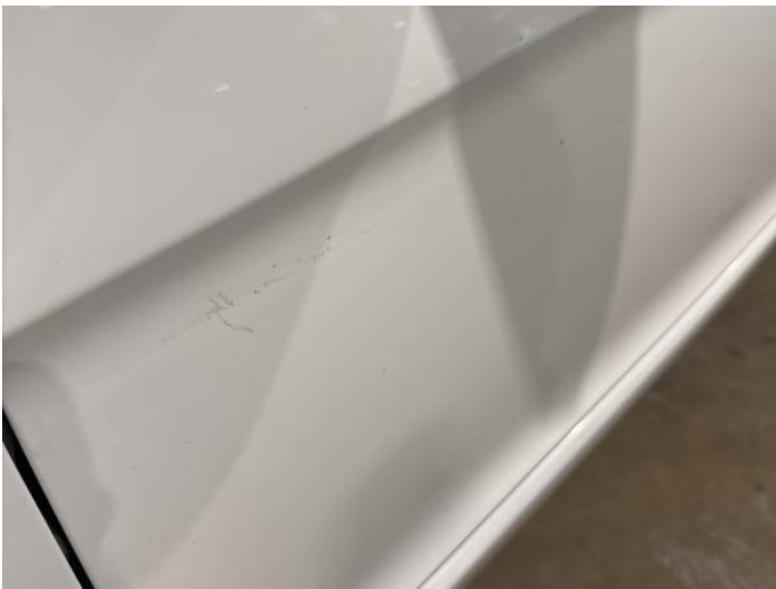
5: Door nsf Scratched Over 25mm Thru Paint
